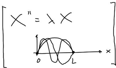
$\rightarrow \underline{X_n(x) = B_n \sin\left(\frac{n\pi x}{L}\right); n = 1, 2, 3, \dots}$
