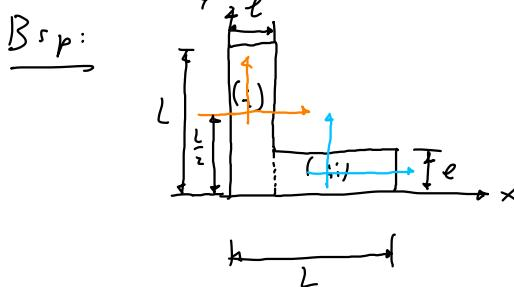
$$\begin{aligned} I_x &= I_{x(1)} + I_{x(2)} \quad |_{\text{Steiner}} \\ I_{x(1)} &= \frac{e L^3}{12} + \underbrace{\overline{L e \left(\frac{L}{2}\right)^2}}_{\text{Steiner}} = \frac{L^3 e}{3} \\ I_{x(2)} &= \underbrace{\frac{(L-e)e^3}{12}}_{\text{Steiner}} + (L-e)e \left(\frac{e}{2}\right)^2 \\ &= \frac{e^3(L-e)}{3} \end{aligned}$$
